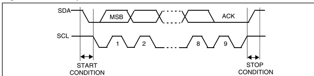
Acknowledge may be enabled or disabled by software. The I<sup>2</sup>C interface addresses (7-bit/10-bit and/or general call address) can be selected by software.
