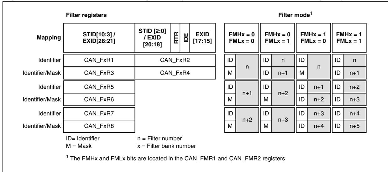
Figure 145. 8-bit filter bank configuration (FSCx bits = 0b00 in CAN\_FCRx register)
