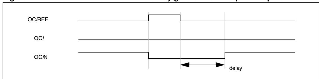
The deadtime delay is the same for each of the channels and is programmable with the DTG bits in the  $TIM1\_DTR$  register. Refer to [Section 17.7.31: Deadtime register \(TIM1\\_DTR\) on page 208](#) for delay calculation.
