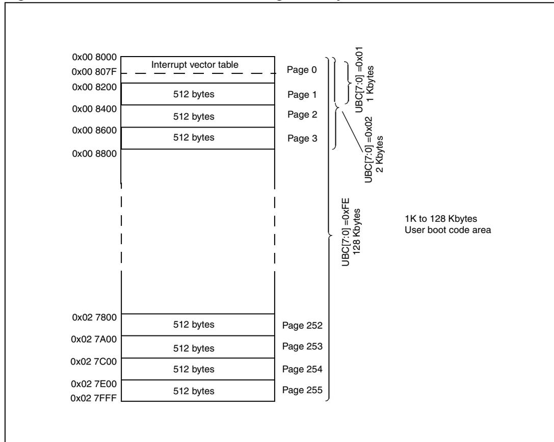
1. UBC[7:0] = 0x00 means no user boot code area is defined. Refer to the datasheets for the description of the UBC option byte.
