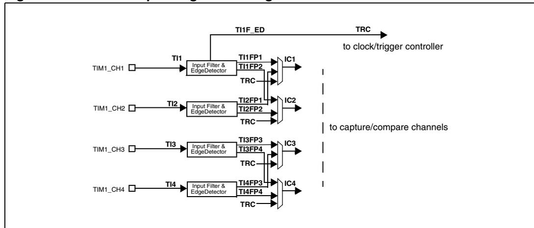
Figure 61 shows how the input stage samples the corresponding TI/ input to generate a filtered signal TI/F. Then, an edge detector with polarity selection, generates a signal (TI/FPn) which can be used as trigger input by the clock/trigger controller or as the capture command. The signal is prescaled before entering the capture register (IC/PS).
