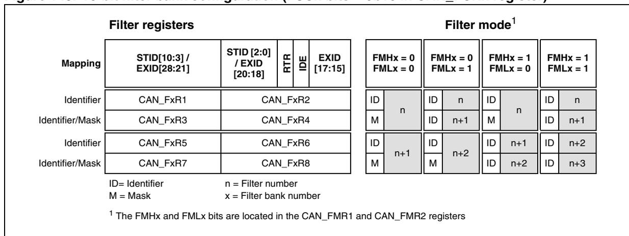
Figure 144. 16/8-bit filter bank configuration (FSCx bits = 0b01 in CAN\_FCRx register)
