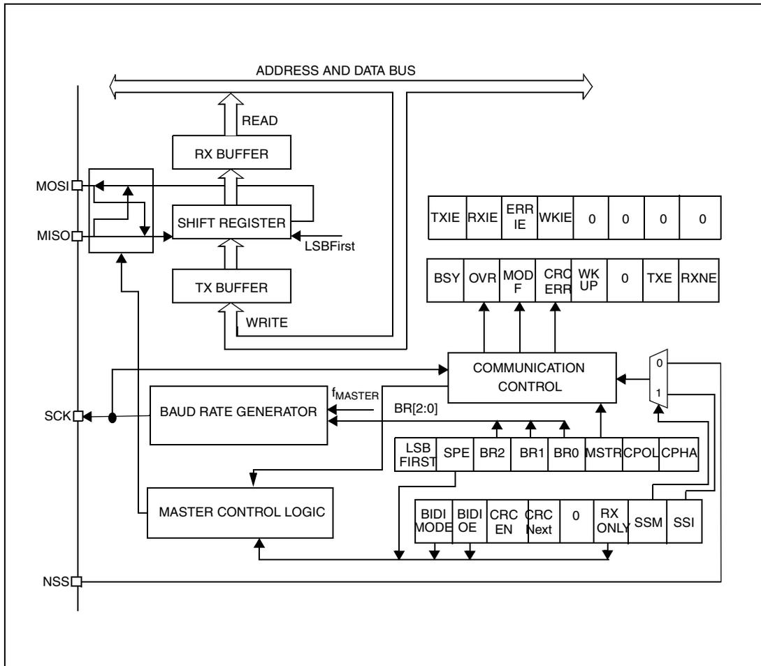
The SPI is connected to external devices through four pins:
