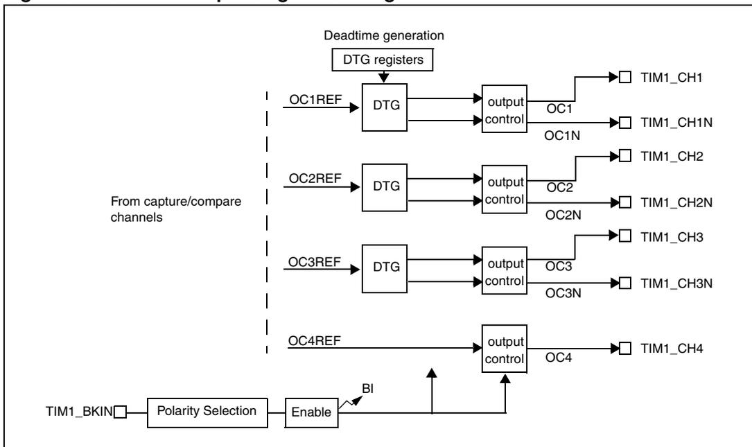
Figure 65. Detailed output stage of channel with complementary output (channel 1)
