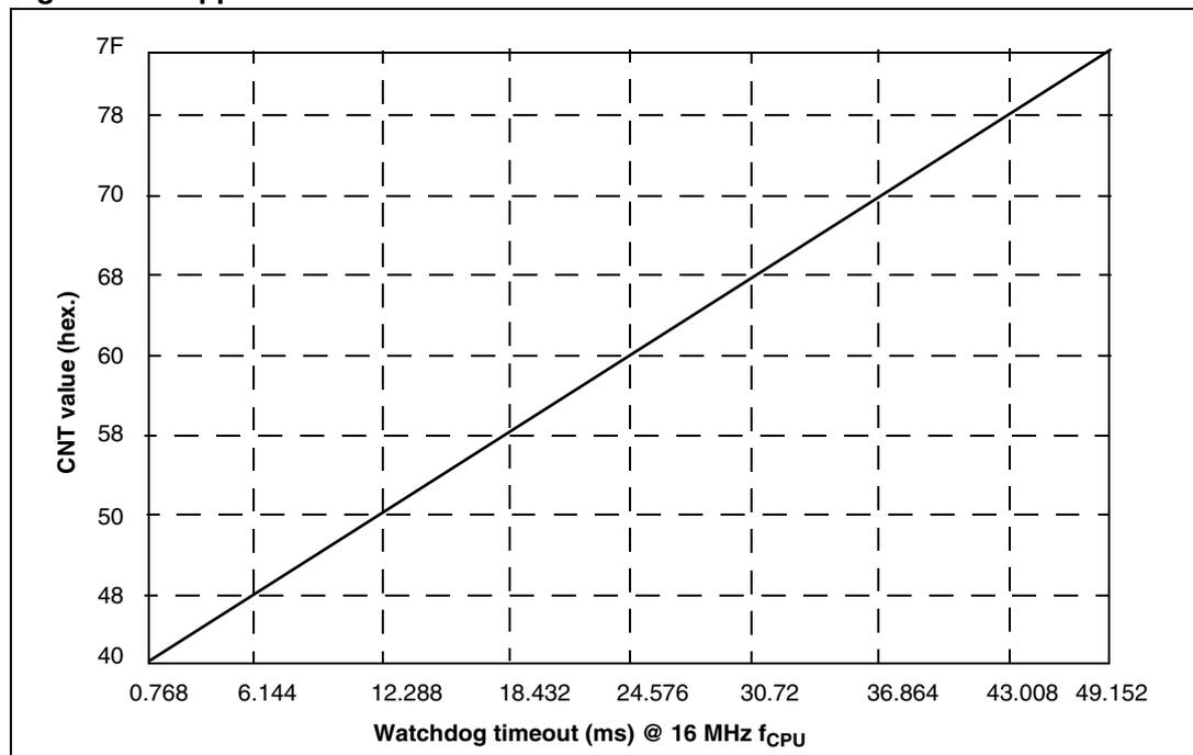
Figure 27. Window watchdog timing diagram
