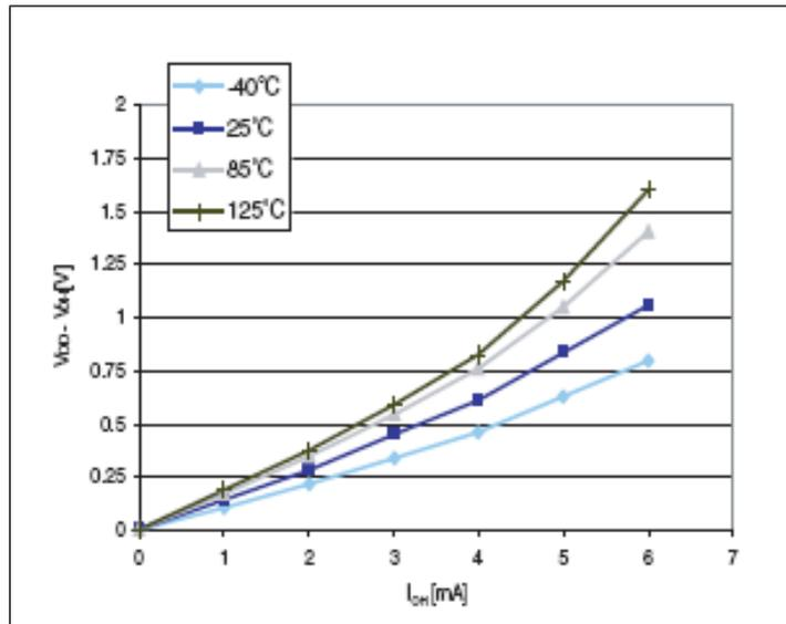
Figure 32: Typ.  $V_{DD} - V_{OH} @ V_{DD} = 3.3\text{ V}$  (standard ports)
