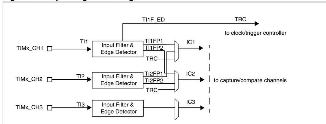
**Figure 83. Input stage of TIM 2 channel 1**
