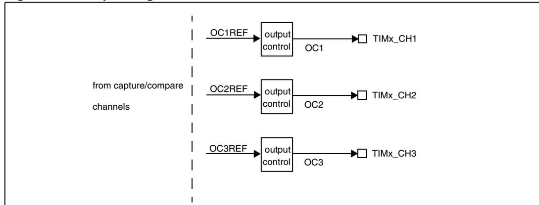
The output stage generates an intermediate waveform which is then used for reference: OCxREF (active high). Polarity acts at the end of the chain (see [Figure 85](#)).
