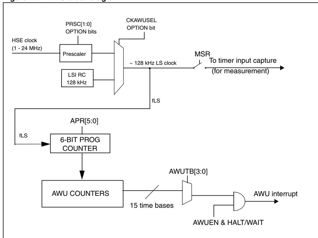
*Note:* The LS clock source is selected by programming the CKAWUSEL option bit as explained in the clock controller chapter.
