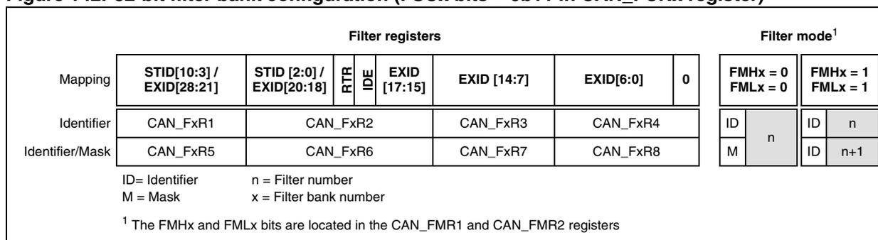
**Figure 143. 16-bit filter bank configuration (FSCx bits = 0b10 in CAN\_FCRx register)**
