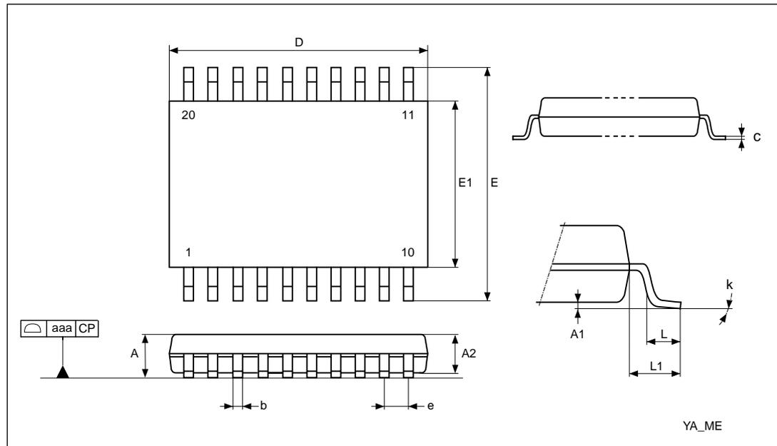
Table 56: 20-pin, 4.40 mm body, 0.65 mm pitch mechanical data
