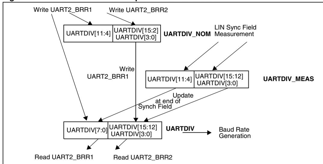
Figure 131. UARTDIV read / write operations when LDUM = 1
