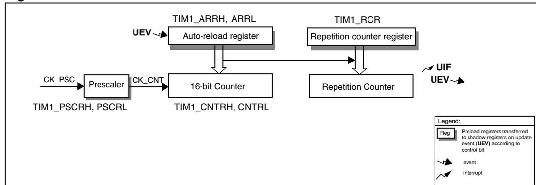
The 16-bit counter, the prescaler, the auto-reload register and the repetition counter register can be written or read by software.
