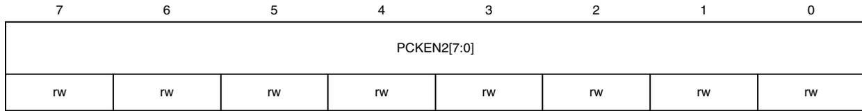
Bits 7:0 **PCKEN2[7:0]**: Peripheral clock enable
