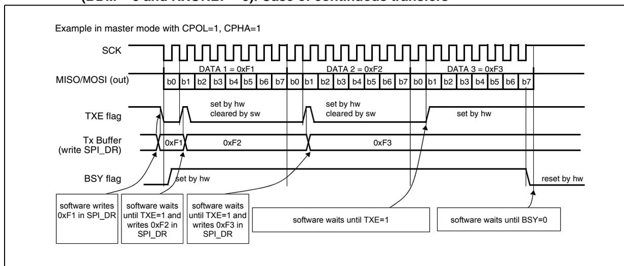
**Figure 95. TXE/BSY in slave transmit-only mode (BDM = 0 and RXONLY = 0).
