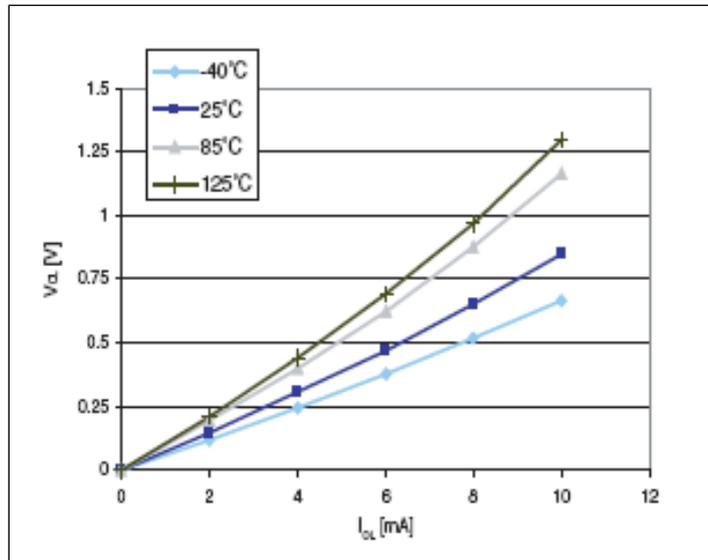
Figure 26: Typ.  $V_{OL}$  @  $V_{DD} = 3.3\text{ V}$  (standard ports)
