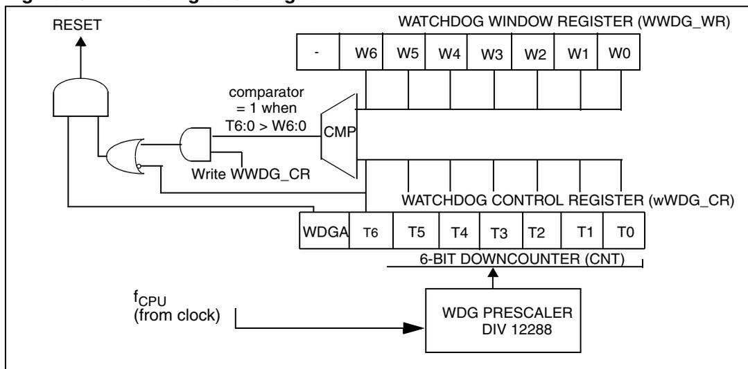
The application program must write in the WWDG\_CR register at regular intervals during normal operation to prevent an MCU reset. This operation must occur only when the counter value is lower than the window register value. The value to be stored in the WWDG\_CR register must be between 0xFF and 0xC0 (see [Figure 26](#)):
