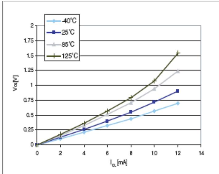
Figure 29: Typ.  $V_{OL}$  @  $V_{DD} = 5\text{ V}$  (high sink ports)
