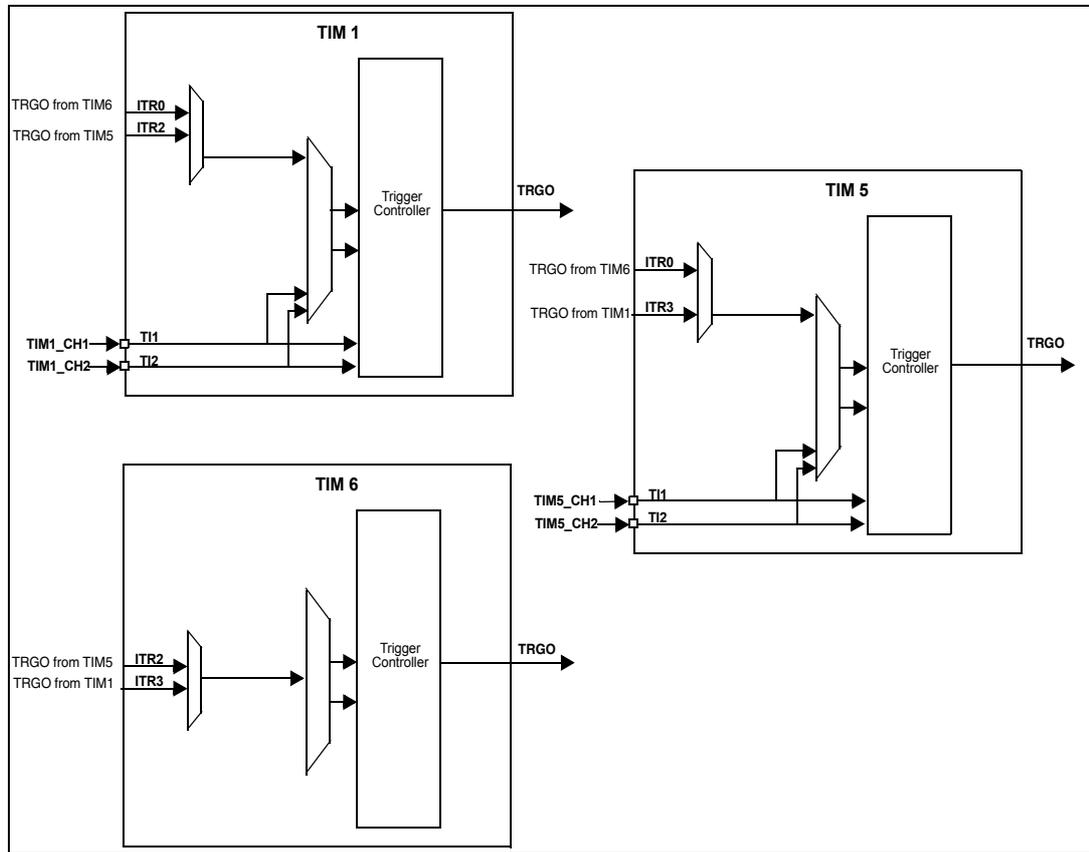
Figure 51 presents an overview of the trigger selection and the master mode selection blocks.
