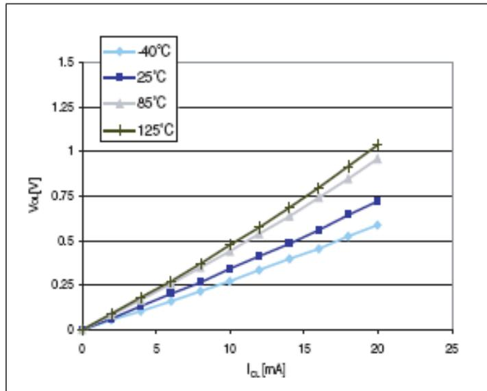
Figure 30: Typ.  $V_{OL}$  @  $V_{DD} = 3.3$  V (high sink ports)
