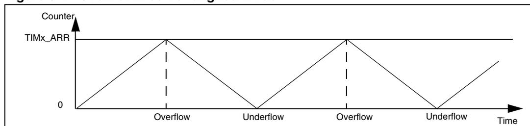
If the timer has a repetition counter (as in TIM1), the UEV is generated after up and down counting and repeated for the number of times programmed in the repetition counter register (TIM1\_RCR). Otherwise, the UEV is generated at each counter overflow and at each counter underflow.
