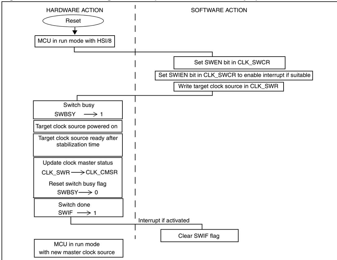
Figure 16. Clock switching flowchart (manual mode example)
