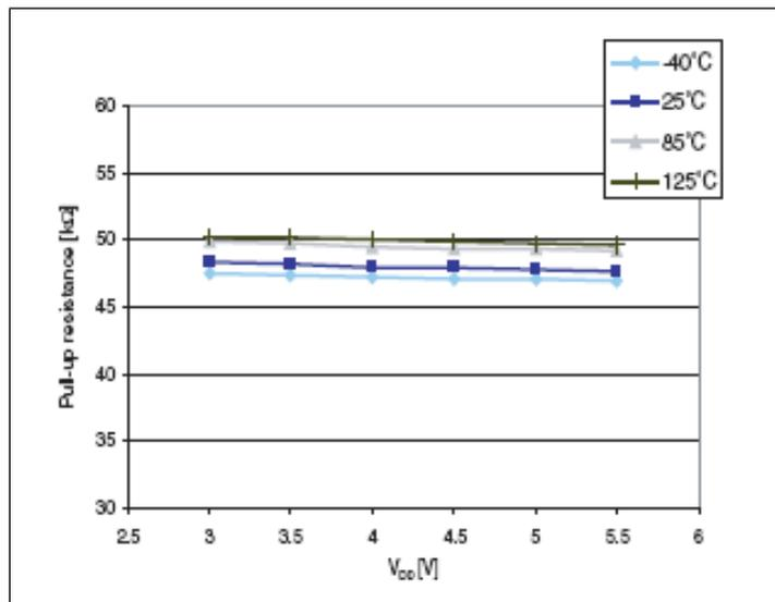
Figure 24: Typical pull-up current vs  $V_{DD}$  @ 4 temperatures
