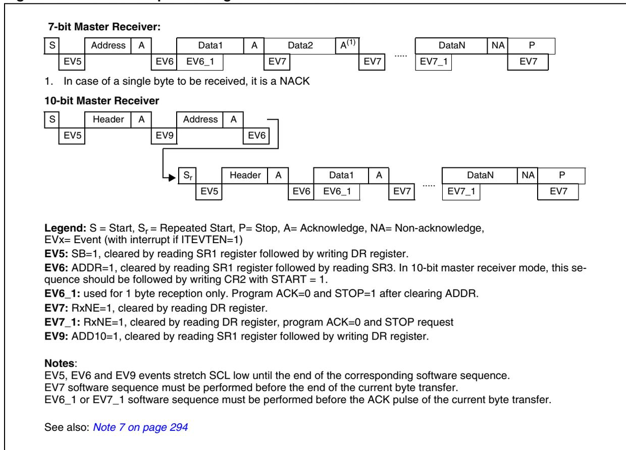
1. If the DR and shift registers are full, the next data reception (I<sup>2</sup>C clock generation for slave) is performed after the EV7 event is cleared. In this case, EV7 does not overlap with data reception.
