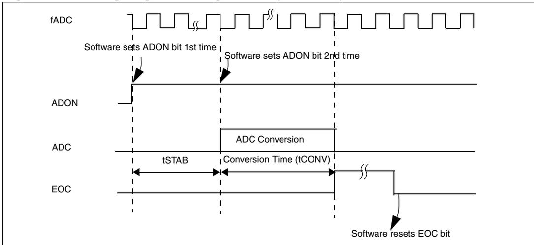
**Figure 158. Timing diagram in continuous mode (CONT = 1)**
