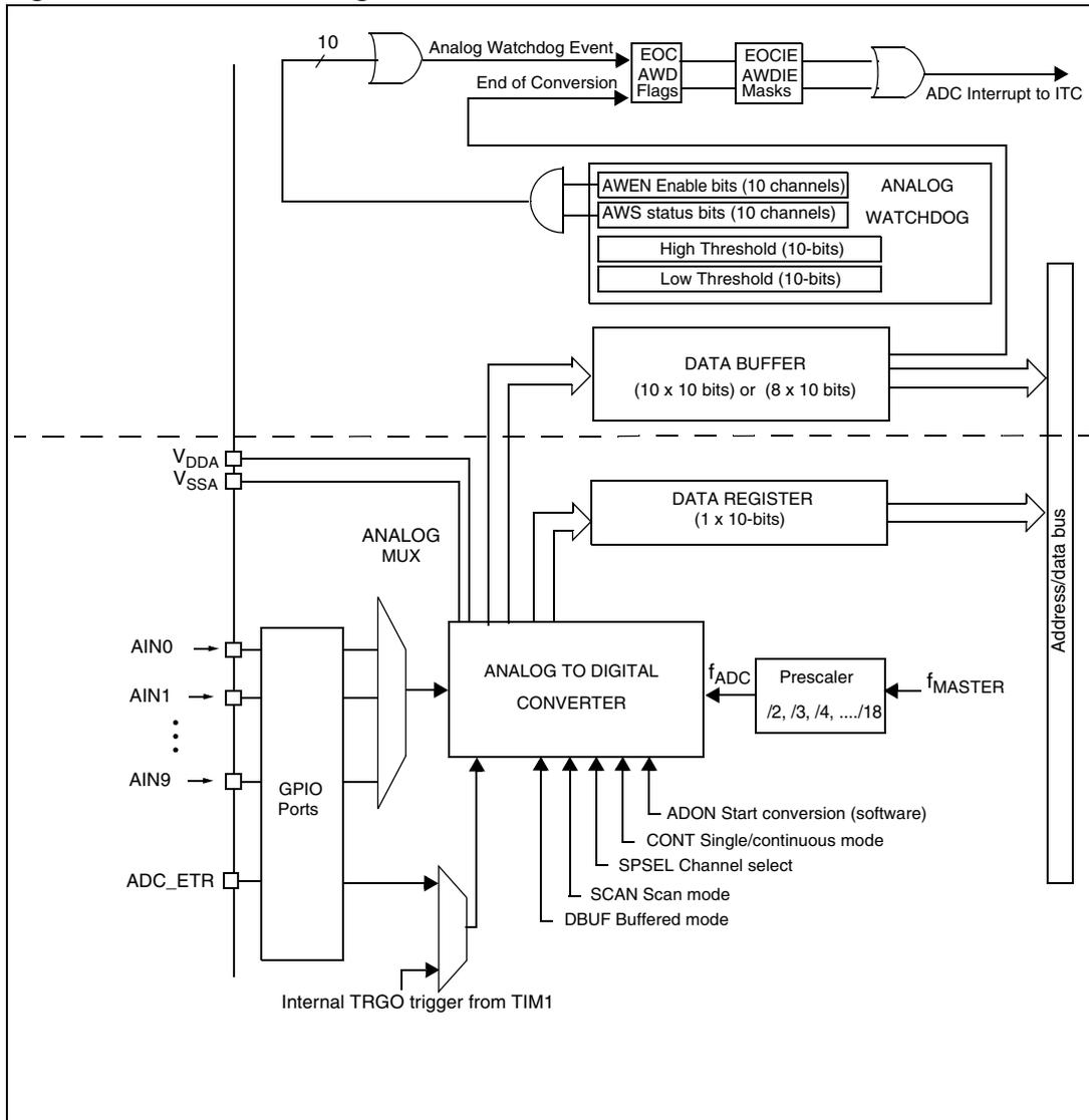
Figure 155. ADC2 block diagram
