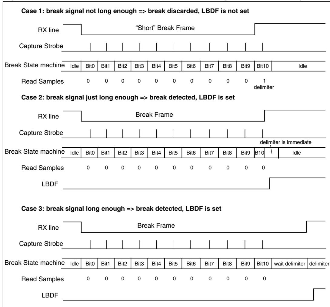
**Figure 125. Break detection in LIN mode vs framing error detection**
