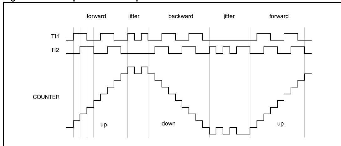
Figure 78 gives an example of counter behavior when IC1 polarity is inverted (same configuration as Figure 77 except that CC1P = 1).
