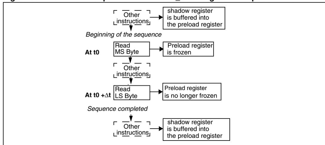
[Figure 59](#) shows the sequence for reading the  $CCRi$  registers in the 16-bit timers. This buffered value remains unchanged until the 16-bit read sequence is completed.
