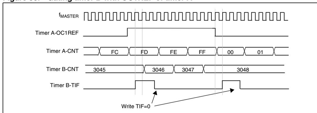
In [Figure 53](#), the timer B counter and prescaler are not initialized before being started. Therefore, they start counting from their current value. It is possible to start from a given value by resetting both timers before starting timer A. In this case, any value can be written in the timer counters. The timers can easily be reset by software using the UG bit in the TIMx\_EGR registers.
