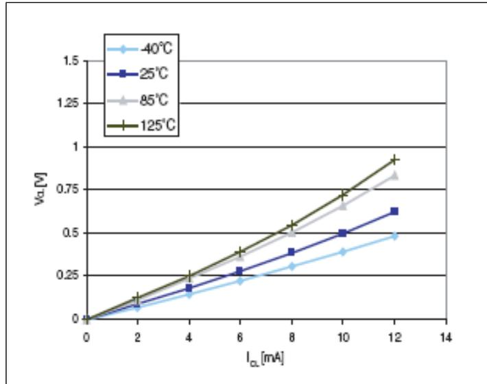
Figure 31: Typ.  $V_{DD} - V_{OH}$  @  $V_{DD} = 5$  V (standard ports)
