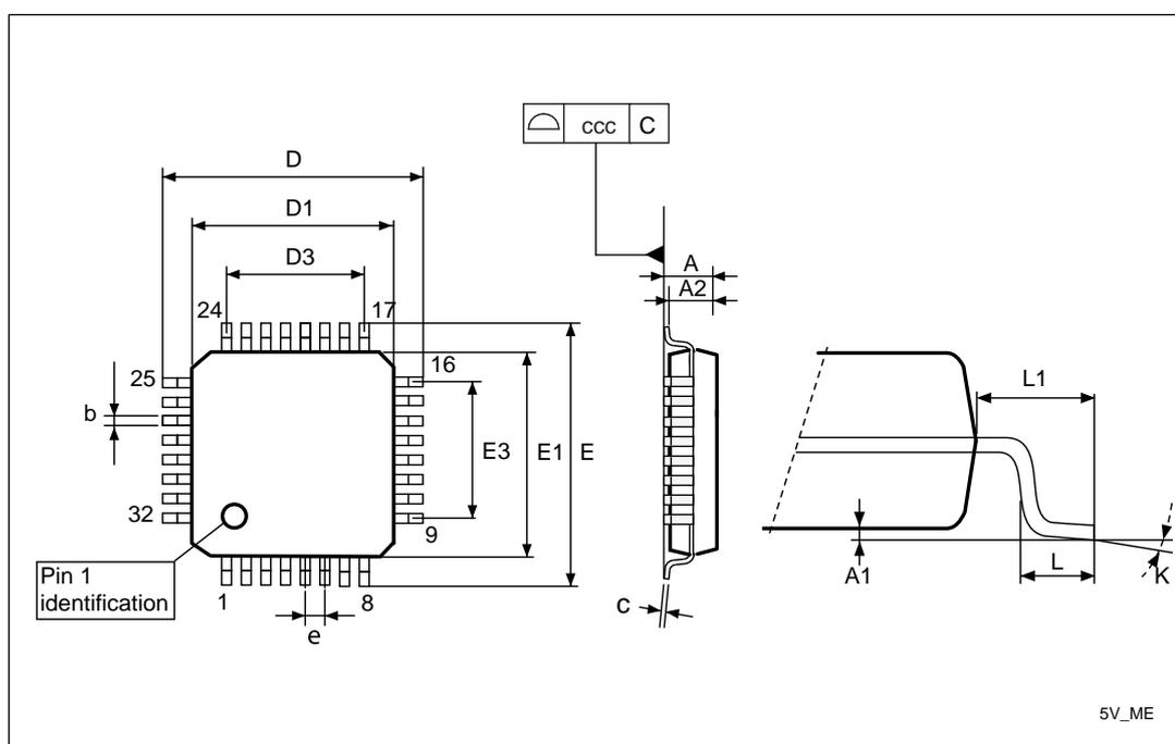
Table 52: 32-pin low profile quad flat package mechanical data
