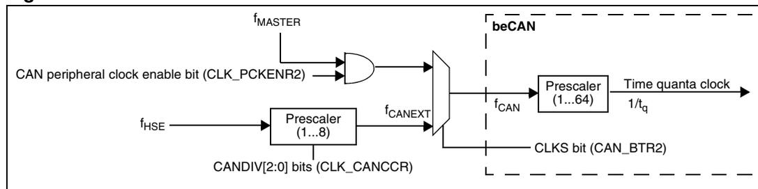
The frequency of the external clock  $f_{\text{CANEXT}}$  must be less than that of the CPU clock ( $f_{\text{CPU}}$ ).
