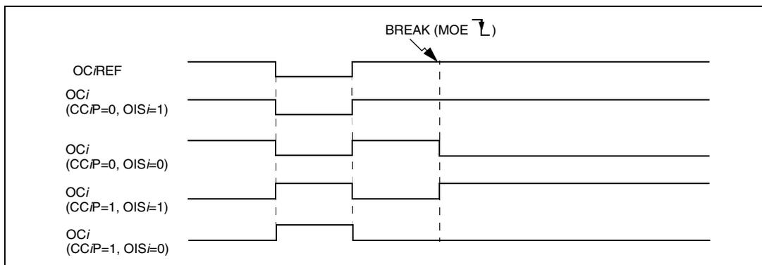
Figure 75 shows an example of behavior of the complementary outputs (TIM1 only) in response to a break.
